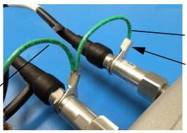
Ground wire from antenna connector 1 to 2
