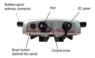
Weatherproof caps protect the connectors on the bottom panel. Rubber caps cover the antenna connectors.
