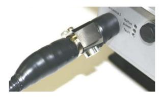
8. Wrap a second layer of electrical tape over the first layer of electrical tape.
