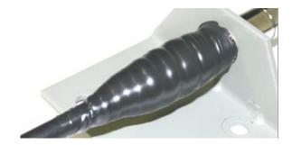
8. Wrap a second layer of electrical tape over the first layer of electrical tape. The antenna connector is ready for installation in an outdoor environment.
