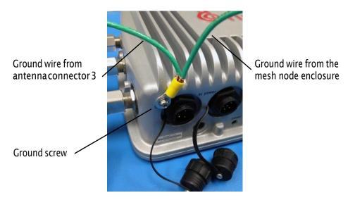
6. Crimp the lug that holds the wire from antenna connector 3 and the enclosure.
