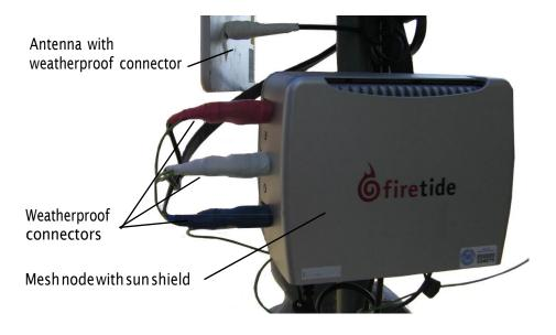
**Best practice:** You can use colored tape for easy identification of the connectors from the mesh node to the antenna.
