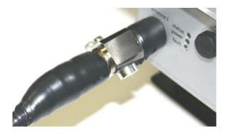
8. Wrap a second layer of electrical tape over the first layer of electrical tape. The lightning arrestor connections are ready for installation in an outdoor environment.
