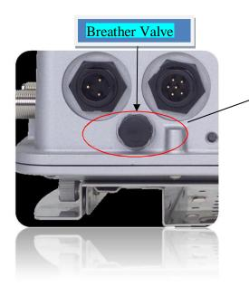
The reset button is behind the breather valve, so removal of the breather valve is required in order to reset the 7020 mesh node.
