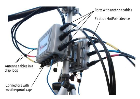
The next picture shows a correctly installed mesh node, with a drip loop and weatherproof connections.
