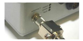
4. Wrap a layer of electrical tape (sticky side out) over the arrestor to node connector and wrap approximately 1 inch (2.5 cm) of cable. Overlap the tape by 40% with each turn.
