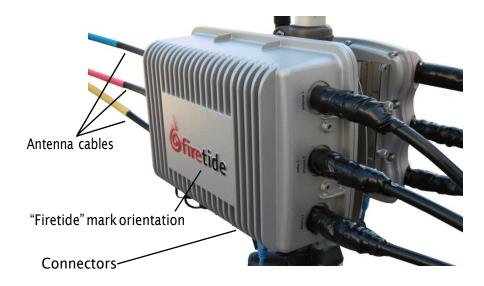
The installation is correct if the device does not move side to side easily, the "Firetide" mark is oriented correctly, and the connectors are oriented to the ground.
