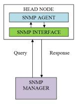
When the SNMP manager is directly connected to a mesh node (head node), the communication sequence is:
