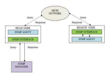
When the SNMP manager is indirectly connected to a mesh node (remote node), the communication sequence is:
