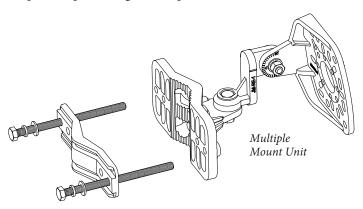
Mounting Clamp Saddle with M8x140 bolts, flat and lock washers
