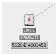
The next image shows the HotView Pro icon for a 5020-E with a broken (down) radio link. The link line color is red. A red circle with an 'X' is on the device, and a yellow circle with a red exclamation symbol is next to the device icon.
