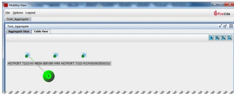
In an aggregate view, groups of similar devices appear in a cloud with a number that represents the number of devices. For example, if you have 10 mobile nodes all attached to the same HotPort static mesh node and all 10 are up and running, a green cloud with the number 10 appears with a dotted line to represent the link. Reducing the number of icons on the monitor makes it easier to analyze the state of the network during video or data offload tasks.
