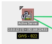
**Gateway interface.** A gateway interface mode has one connection to a gateway server and connections to other mesh or 5020-Es. The next image shows a gateway interface.
