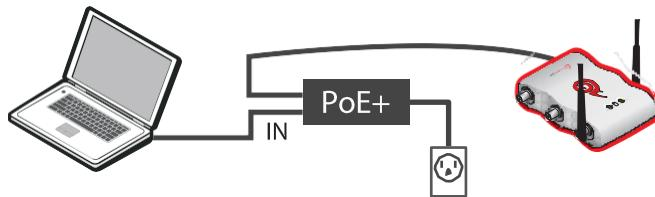
The access point boots in 1.5 to 2 minutes. The power LED glows steady and the 2.4G LED blinks.
