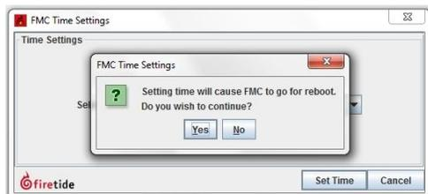
The FMC device reboots and then appears in the Mobility view. If the network has a redundant FMC, both FMC devices reboot and sync.
