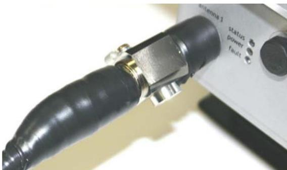
8. Wrap a second layer of electrical tape over the first layer of electrical tape. The lightning arrester connections are ready for installation in an outdoor environment.
