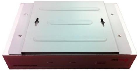
5. Attach the bracket to the mesh node with the four screws from the mount kit.
