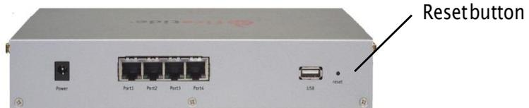
Do a reset when you remove a device from the field or when communication with a device is lost.
