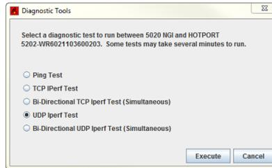
**Note:** Iperf tests flood a link with as much traffic as it can carry. This can disrupt other traffic on the mesh. Iperf sends a large, fixed amount of traffic. If iperf cannot complete the transfer in a fixed period of time, it stops. If you receive a failure message, run the test again. If the test fails consistently, substantial interference exists on the RF link.
