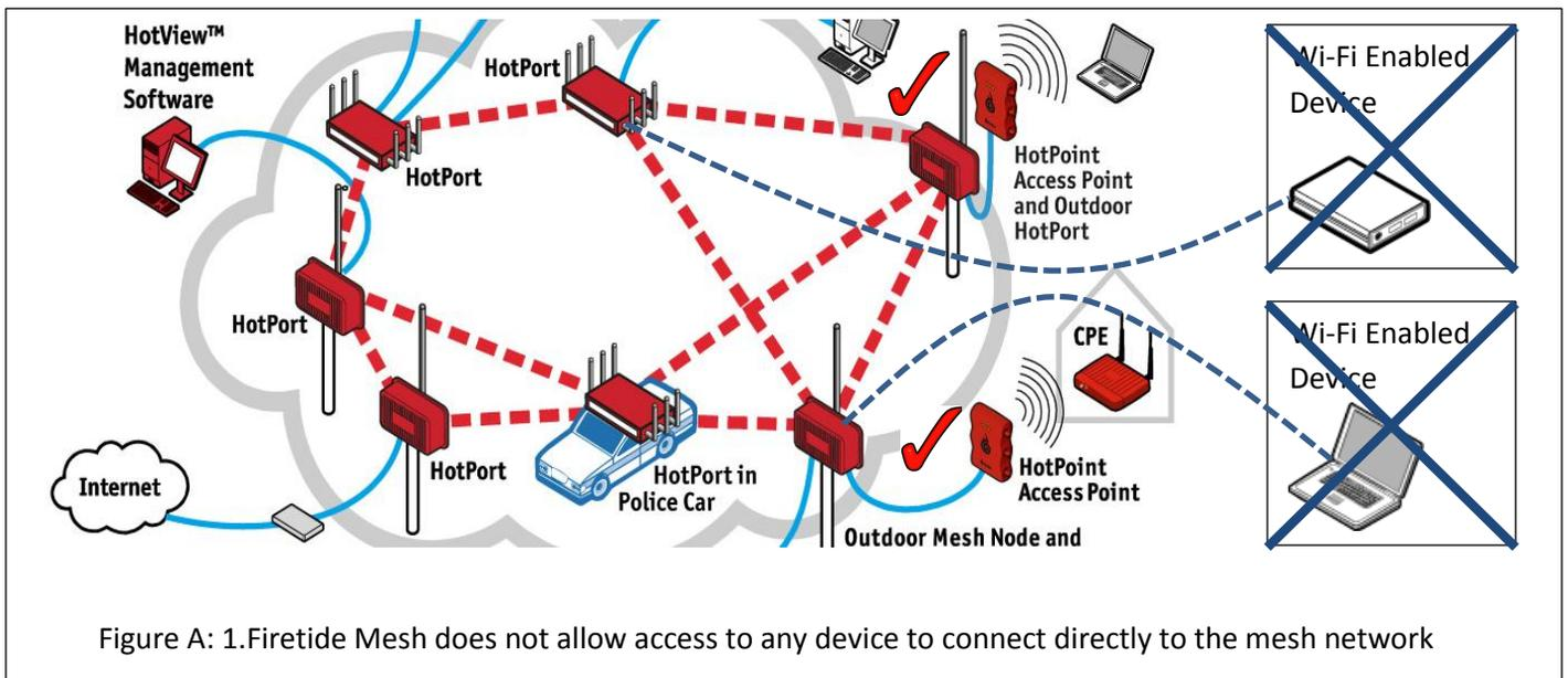
1. Firetide wireless infrastructure mesh provides reliable and secure connectivity critical for bandwidth intensive applications and wireless networks. Firetide mesh uses proprietary protocols to communicate between the Firetide HotPort mesh nodes. This protocol is insusceptible to other Wi-Fi enabled devices. Hence, any device (including laptops, smartphones, tablets, and similar Wi-Fi devices) other than the Firetide HotPort mesh node cannot connect or communicate directly to the Mesh.
