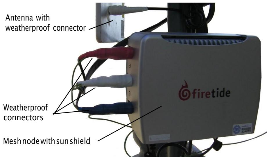
**Best practice:** You can use colored tape for easy identification of the connectors from the mesh node to the antenna.
