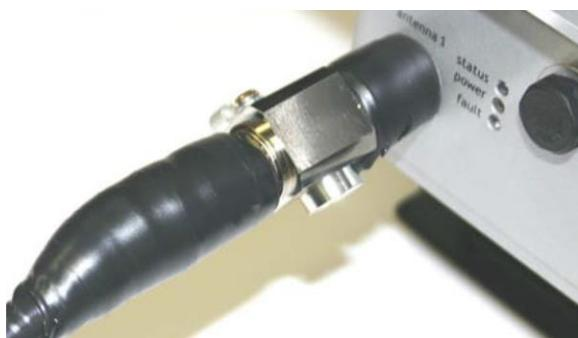
8. Wrap a second layer of electrical tape over the first layer of electrical tape.
