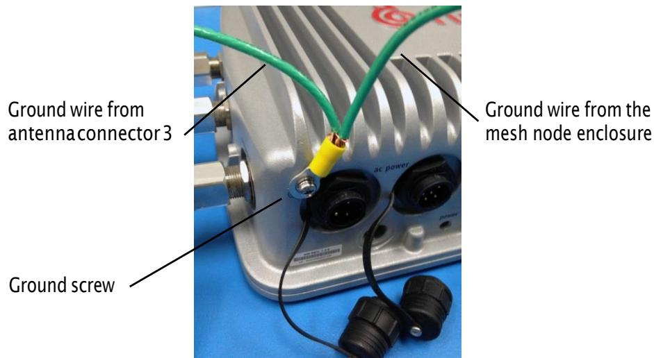
6. Crimp the lug that holds the wire from antenna connector 3 and the enclosure.
