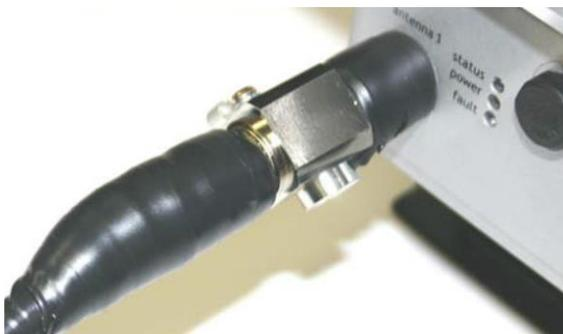
8. Wrap a second layer of electrical tape over the first layer of electrical tape. The lightning arrester connections are ready for installation in an outdoor environment.
