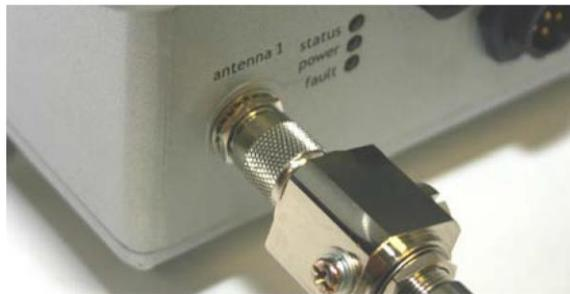
4. Wrap a layer of electrical tape (sticky side out) over the arrestor to node connector and wrap approximately 1 inch (2.5 cm) of cable. Overlap the tape by 40% with each turn.
