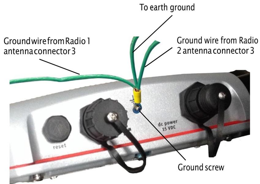
6. Crimp the lug that holds the wire from antenna connector 3 and the enclosure.
