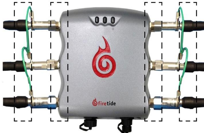
**Best practice:** You can use colored tape for easy identification of the connectors from the mesh node to the antenna.
