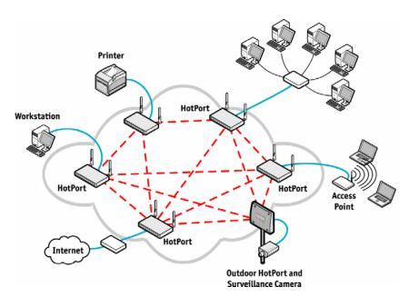
A "mezzanine" mesh network cloud as a DMZ connected to another network
