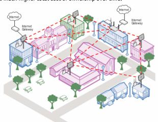
A mesh network interfacing with access points and connecting to an enterprise/service provider network
