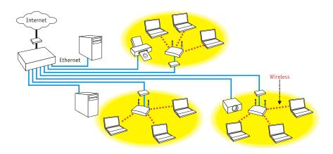
The substantial wiring (links) required to implement a "wireless" network
