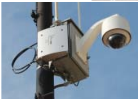
The wireless mesh-based video surveillance system has curtailed vandalism of public fountains and other important landmarks in Anderson, S.C.
